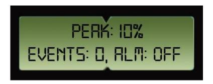
Assuming the cable is attached and properly terminated (the Cable status LED is Green). The LCD will show the Peak and Average sound recorded and the number of recorded events in each window of time as currently set. The alarms will not be latched and the siren will not sound. If there is an "Alarm" the number on the LCD will increment.
