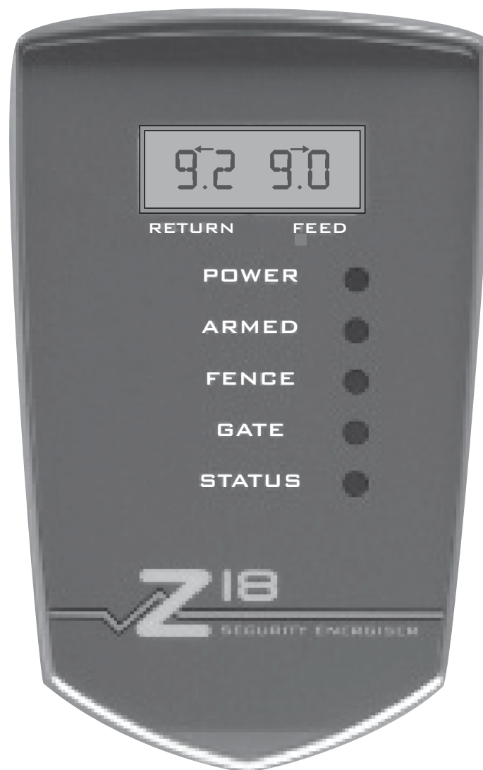
Figure 3: LCD Display and Status LEDs
